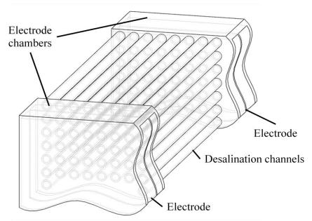
**Figure S6.** Cutaway schematic demonstrating a potential scale-up concept for EPD using multiple channels in parallel. The anodic and cathodic electrode chambers are connected by many desalination channels in parallel. A single pair of electrodes serves the entire device.
