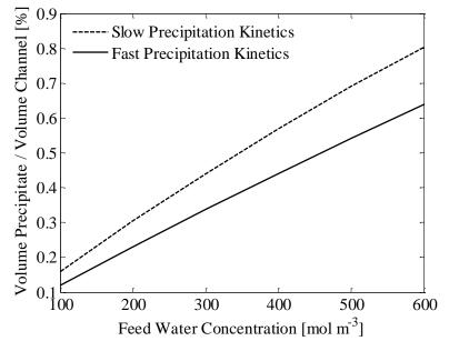
**Figure S2**. Theoretical ratio of precipitate volume to channel volume as a function of feed water concentration (100 to 600 mol  $m^{-3}$  sodium chloride) based on the slow precipitation kinetics
