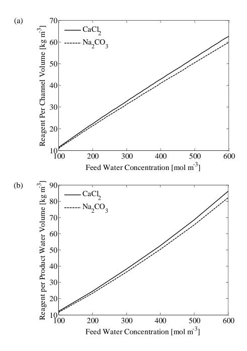
**Figure S3**. Calcium chloride (solid line) and sodium carbonate (dashed line) consumption as a function of feed water concentration (100 to 600 mol  $m^{-3}$  sodium chloride) per volume of channel (a) and per volume of product water (b). We obtain the reagent consumption per volume of product water by dividing reagent consumption per volume of channel by the ratio of product water volume to channel volume as a function of feed water concentration. This ratio is derived in Section SI 5.
