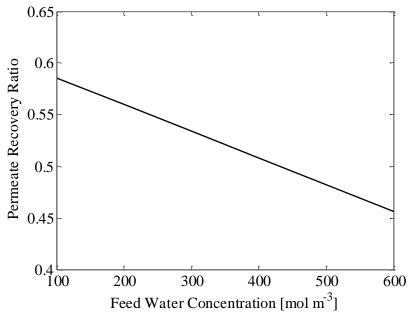
**Figure S4**. Permeate recovery ratio, *PRR*, as a function of feed water concentration. *PPR* varies approximately linearly from 58% to 46% as feed water concentration varies from 100 to 600 mol  $m^{-3}$  sodium chloride. In comparison, typical permeate recovery ratio for sea water reverse osmosis is around 30% to 50 %.<sup>9</sup>
