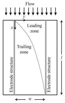
**Figure S7.** Schematic of free flow concept for EPD. The leading zone (feed water zone in anion exchange and sodium carbonate zone in cation exchange) flows between electrode structures, while reagent solutions flow on the other side of porous electrode structures. The flow in the *x*-direction is driven by pressure. A constant potential is applied between the electrode structures, causing shockwaves described in the main text to propagate in the *y*-direction, and trialing zones to develop.
